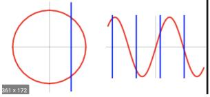
But a circle can be modeled easily with a parametric curve. Use  $I=(0,2\pi), \alpha(t)=(\cos(t),\sin(t))$  Definition Regular curves are curves where at least the second derivative exists and  $\alpha'(t)\neq 0$ . These are curves to which you can fit data. we require  $\alpha'(t)\neq 0$  to guarantee the existence of tangent vectors. Later we also require  $\alpha''(t)\neq 0$  to guarantee the existence of normal vectors.
