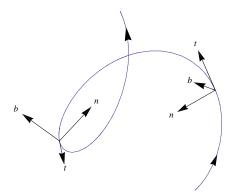
Let  $\alpha: I \to^3$  be a curve parametrized by arc length s such that  $\alpha''(s) \neq 0, s \in I$ . The number  $\tau(s)$  defined by  $\vec{b}'(s) = \tau(s)\vec{n}(s)$  is called the *torsion* of  $\alpha$  at s.
